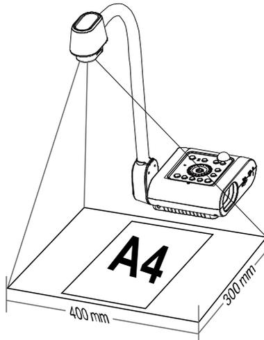
If the camera head is in upright position, press ROTATE on the control panel or remote control twice to rotate the image in 180°.
