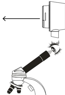
4. Select the appropriate rubber coupler size for the microscope eyepiece and insert it in the microscope adapter.
